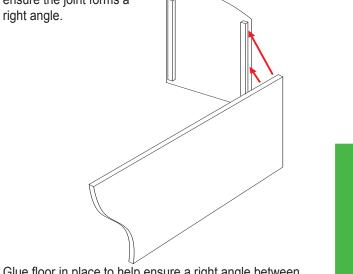
Glue floor in place to help ensure a right angle between the side and end.
